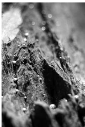
Fig. 13. Shales impregnated with mercury droplets.
